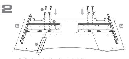
1 Follow the screwing order and screwing in 1/2 depth. Make sure the gap between desktops minimizing. Then screw to the end.
